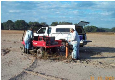
Sampling ground water monitoring wells at a dairy farm
