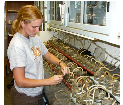
Kelly Nielson connects a temper cell to pressure lines to determine moisture retention.
