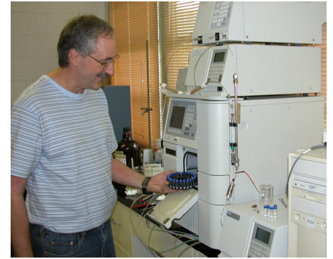
Bill Reve loads a sample into the HPLC to test for organic acids.
