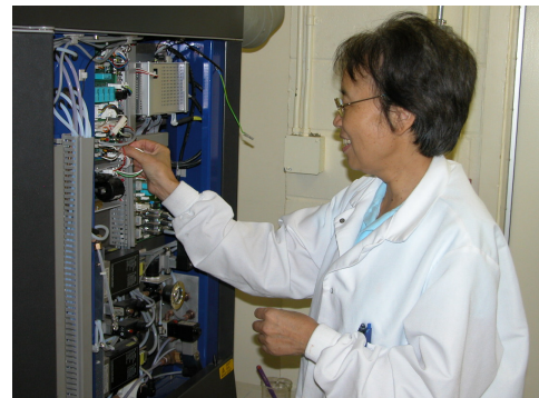
Maintenance of instrumentation insures that our clients receive quality data. Hui X Lu working with one of the lab's ICP instruments for metals analysis.
