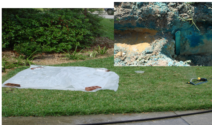
A water-soluble blue marking dye (see blue coloration of turf near the plot stakes) was applied to several areas in the lawn, and then irrigated for various lengths of time. The plastic tarp was used to protect the dyed areas not requiring a particular irrigation. Insert: The blue dye showed that water moved deeper in the sandy soil (right) compared with the clay soil (left), (If excessive water was applied, especially to the sandy soil, then the dye moved below the root zone)
