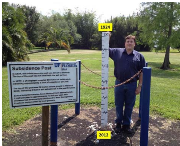
Subsidence post located at Everglades REC near Belle Glade, FL that was driven to bedrock in 1924. The top of the post was at the soil surface in 1924, and approximately 6 feet and 3 inches of soil has been lost up to 2013.
