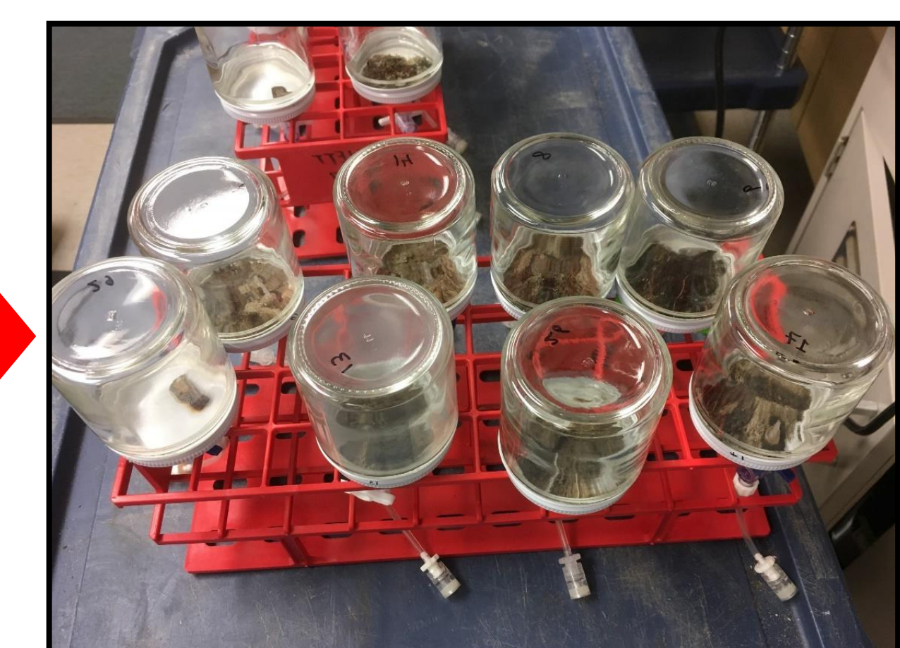
Figure 5. Jars with biocrusts and soil for gas injection/ incubation.
