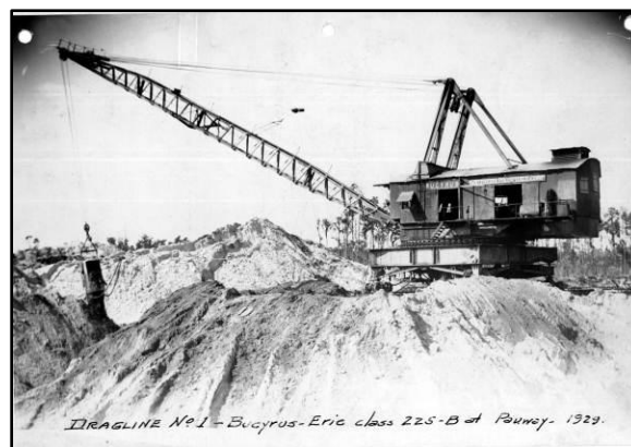
Figure 5. Southern Phosphate Corporation's Bucyrus-Erie class 225B dragline State Archives of Florida, Florida Memory, http://floridamemory.com/items/show/38806
