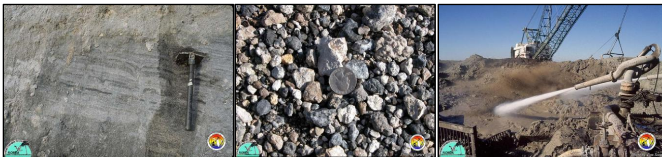
Figure 7. Phosphate matrix (left), larger phosphate pebble (center), pit gun (left). (Florida Geological Survey stock photos—Left and right by Tom Scott; center by Harley Means)
