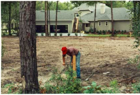
Soil scientists investigate soils in subdivisions to determine depth to high water table and the presence of shrink-swell clays.
