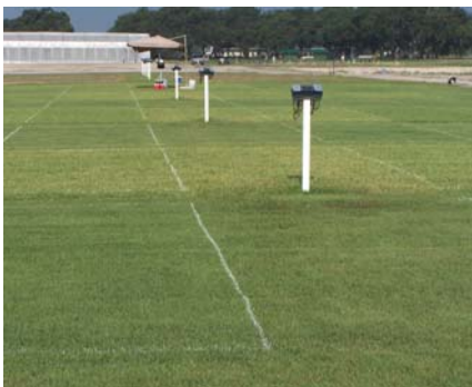
FDEP Environmental Plots—Towers represent collection points for buried lysimeters
