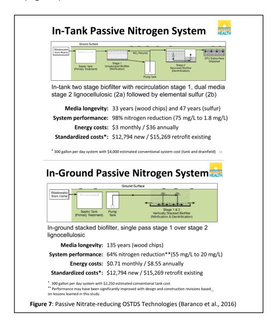
These new passive technologies have been installed and tested under real-life conditions, and have proven to be successful at significantly reducing nitrogen from wastewater, up to 95% (Scott and Armstrong, 2015). However, they are still more expensive to install than conventional systems, which have estimated life time costs of around \$5,542.90 (Scott and Armstrong, 2015). Once the new technologies are approved, policymakers will need
