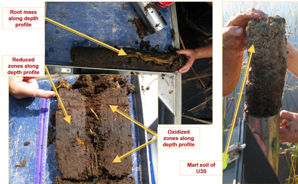
Figure 6. Soil cores collected from the F1, U3R, and U3S sites showing soil composition, root mass, and redox zones along the depth profile.
