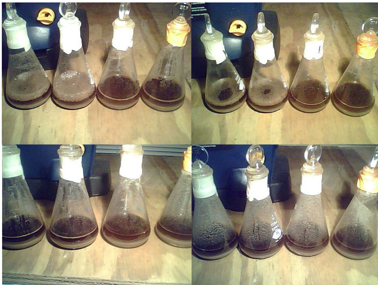
Figure 29: Sequence of unexpected reaction foaming; from upper left, after 2, 3, 5, and 7 days respectively
