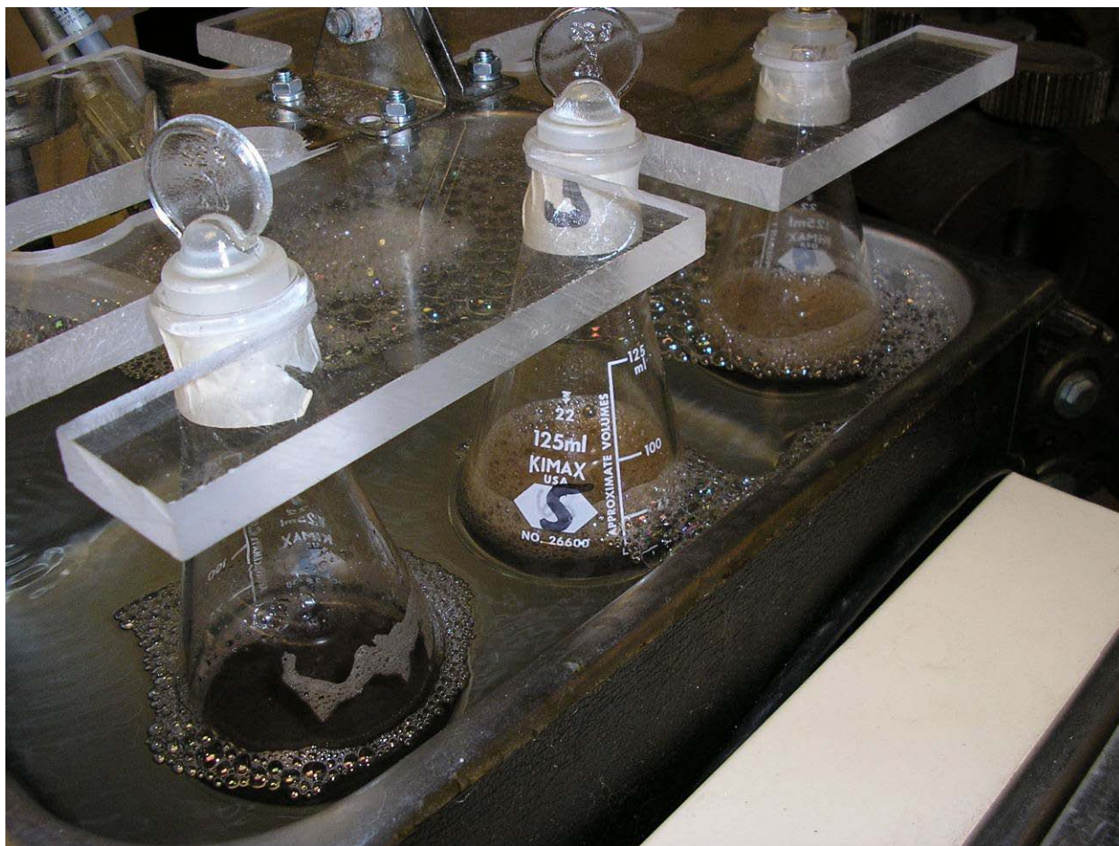
Figure 25: Reaction in progress in ultrasonic bath, note control (no EN Rx) on left
