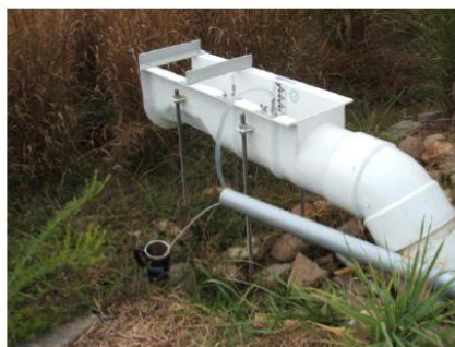
FIGURE 5. FIELD INSTALLATION OF AUTOMATED WATER QUALITY MONITORING INSTRUMENTATION AT CHS BIOFILTER.
