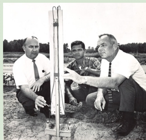
Dr. Luke Hammond (left) with Drs. Saxena (center) and Dr. Charlie Eno (right) looking at the tensiometer to determine soil moisture status. Picture was taken in 1969 at the Suwannee Valley Experiment Station near Live Oak, Florida.
