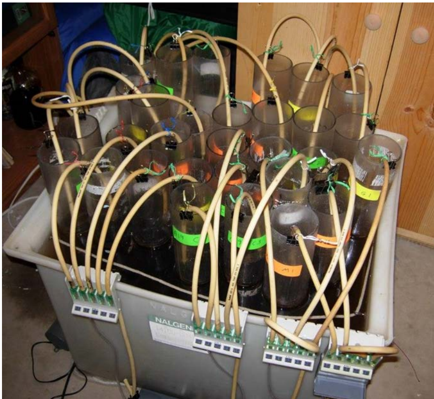
Figure 7. Flooded soil core laboratory set-up showing randomly placed core tubes and mixing apparatus
