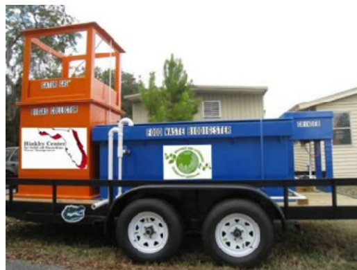
Portable food waste biodigester.
