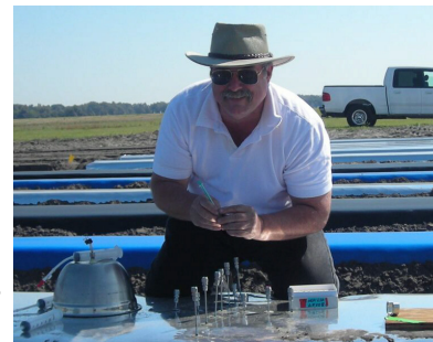
John Thomas sampling the sub-surface soil pore air for pre-crop fumigants
