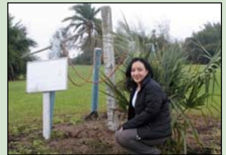
Soil subsidence on muck soils is demonstrated using the subsidence post located near Belle Glade FL. The top of the post was the soil level in 1924.
