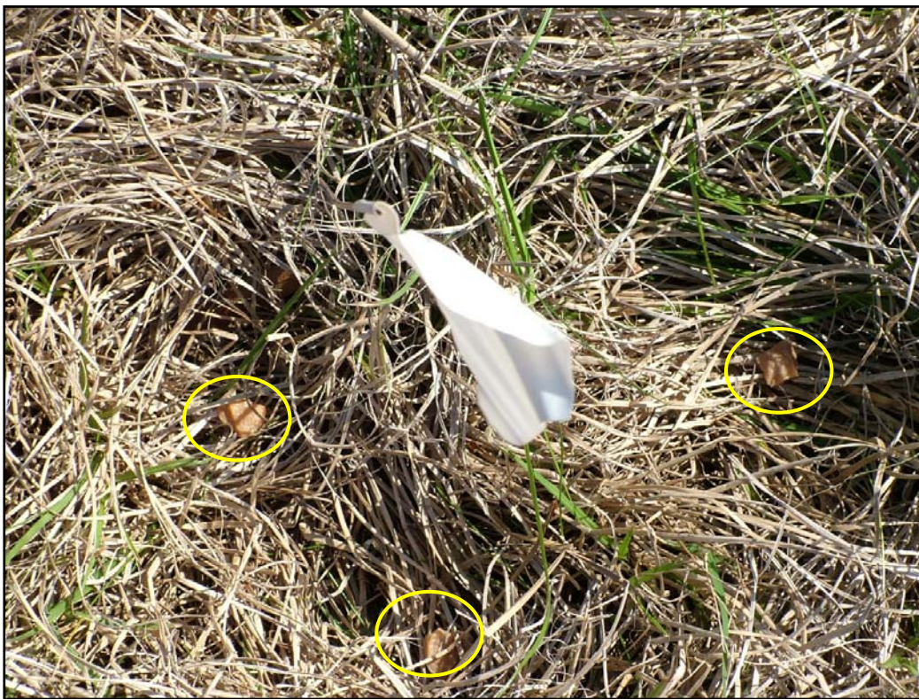
115 Figure 2. Three pieces of Comp-B placed in tampered rings in a demonstration plot.
