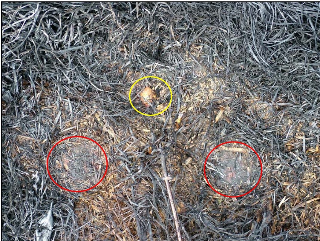
147 Figure 3. Comp-B after a complete burn of a demonstration plot, two pieces combusted 148 (circled red) and one remained (circled yellow).
