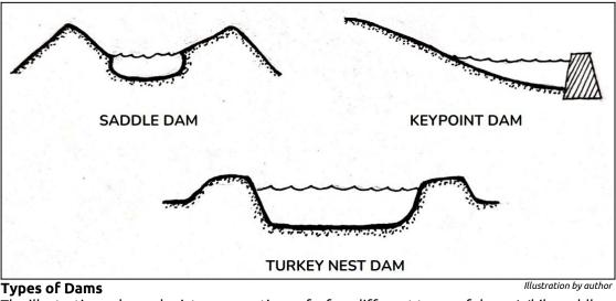
The illustrations above depict cross-sections of a few different types of dams. While saddle dams and keypoint dams can start gravity-fed systems downslope, turkey nest dams on flat land may need to be connected to a pump to move water where needed.
