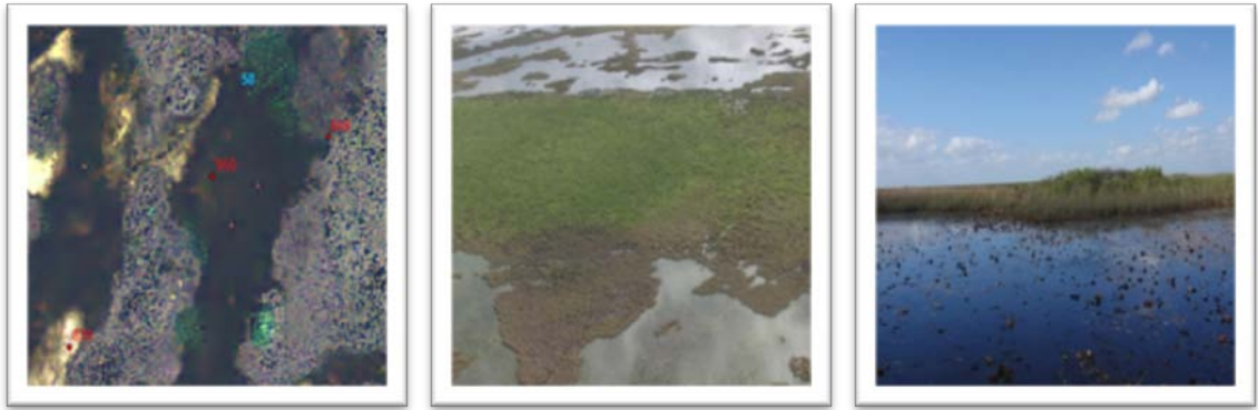
Figure 2-7. Slough – Open Water: Open water is characterized by black color, fine and smooth texture without green dots
