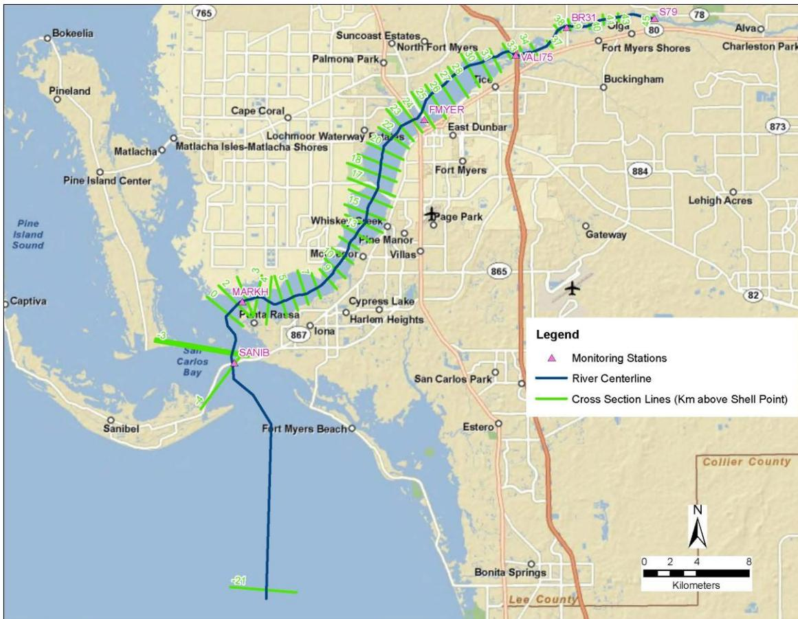
FIGURE 3. Layout of HEC-GeoRAS layers. Sources: Base Map (ESRI Library – US street map layer), Centerline (NHD dataset for subbasin 03090205 with modifications), Cross Sections (Scarlatos 1988 with modification), Monitoring Stations (SFWMD – Salinity Monitoring Stations).
