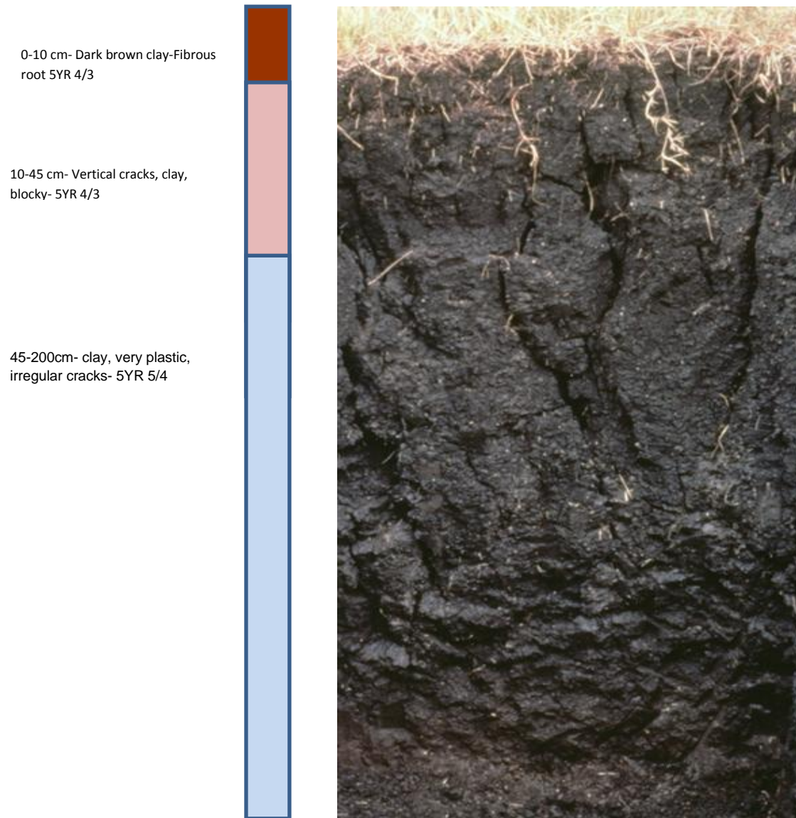
Figure 3. Vertisols profile general characteristics.
