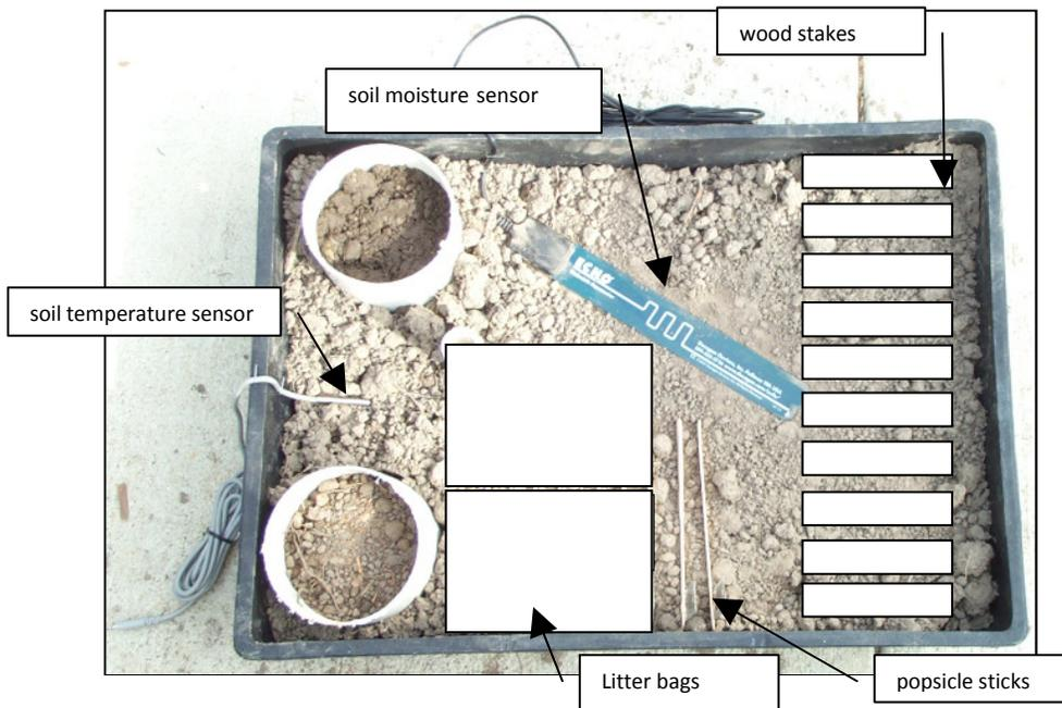
Figure 1. Photograph of experimental tray design, showing the relative locations of PVC collars, sensors, litter bags and wood stakes.
