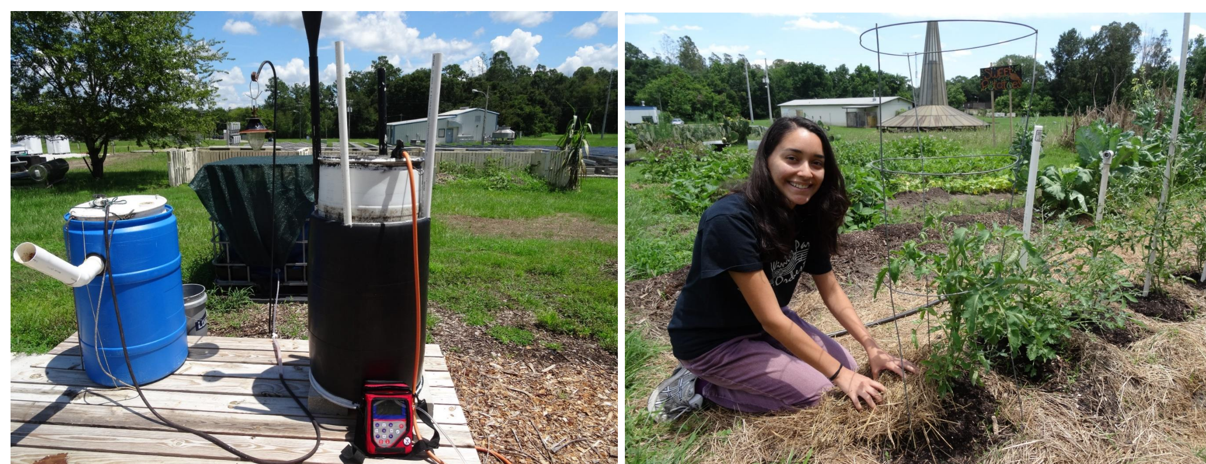
Digesters fed sheep manure at UF-IFAS Bioenergy and Sustainable Technology Laboratory
