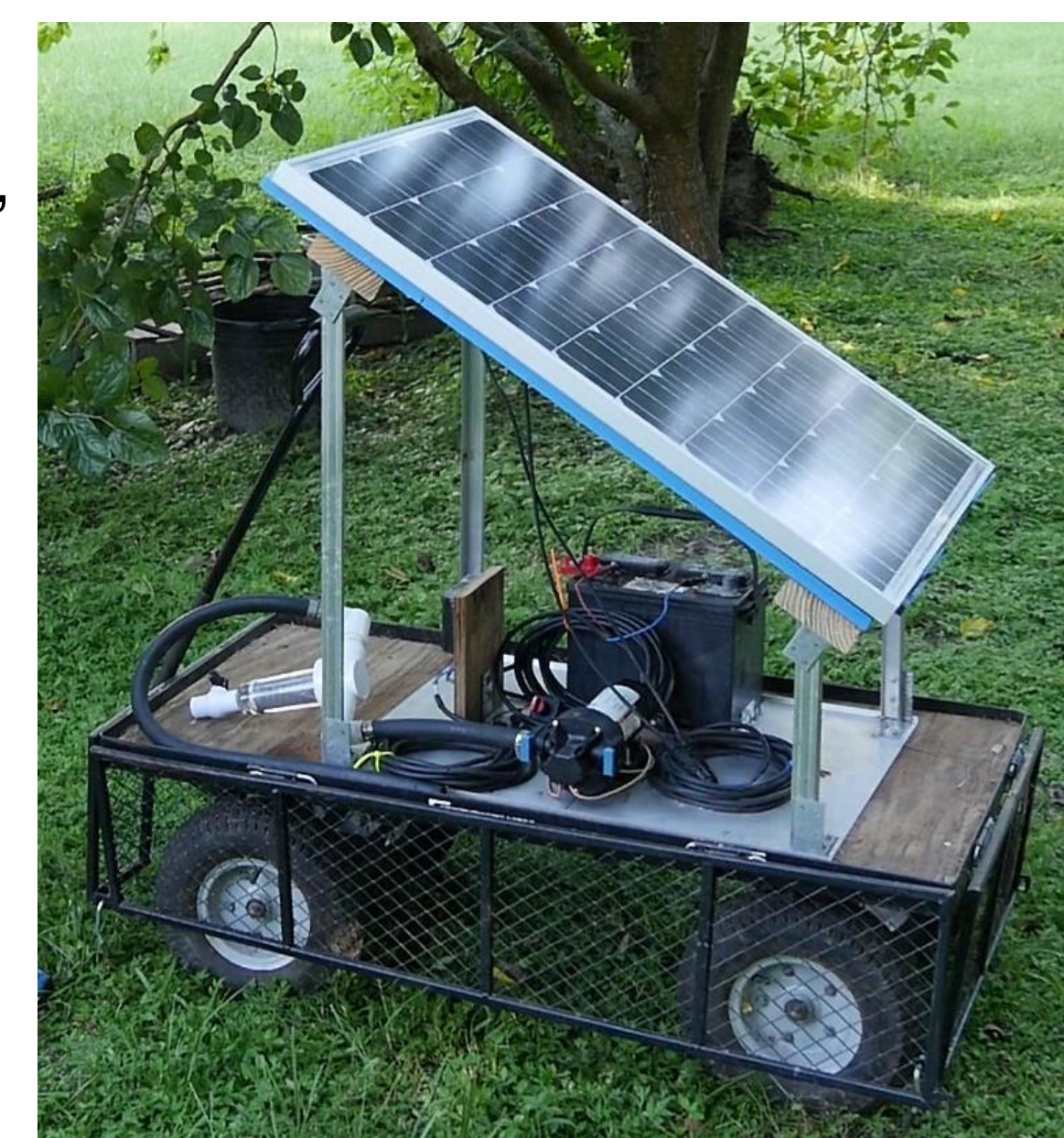
Figure 2. Solar-Powered, Mobile Irrigation Pump.
