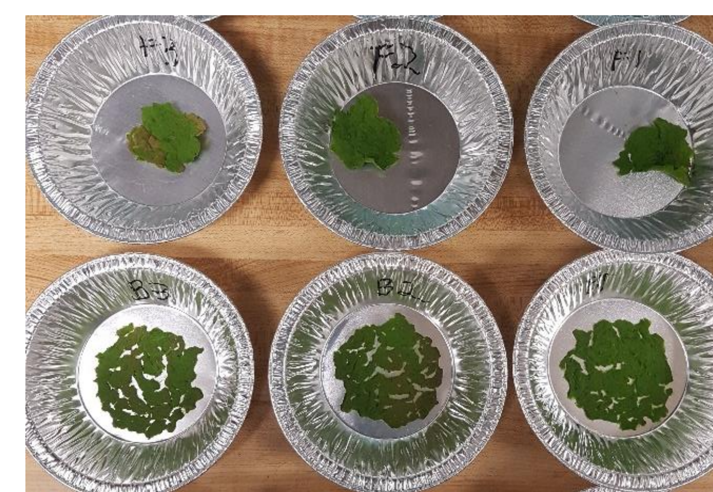
Figure 4: Filament deformation during drying. Top row: intact; Bottom row: fractured
