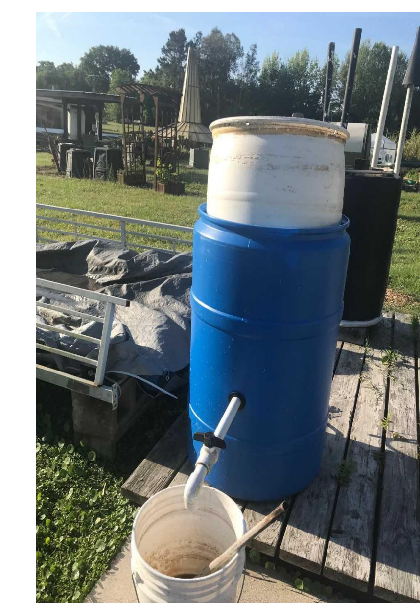
Figure 5: Biogas digester at the BioEnergy and Sustainable Technology Laboratory.
