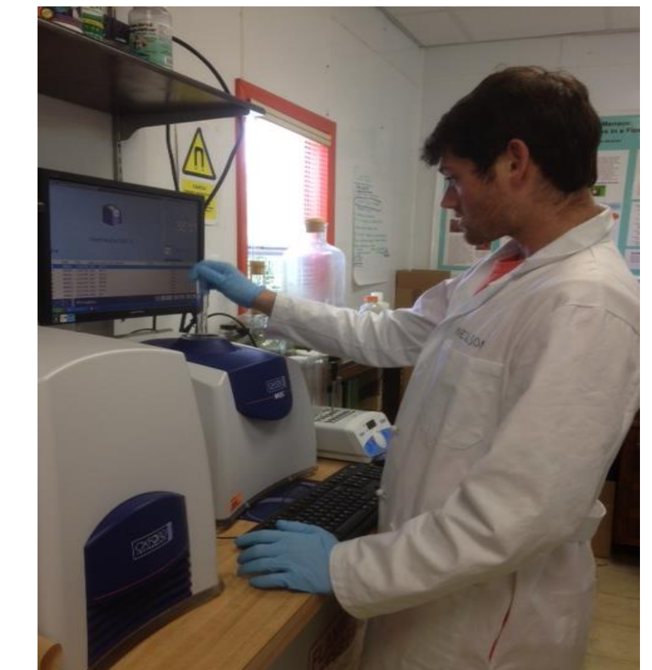
Figure 3. Using nuclear magnetic resonance to determine algal lipid content.
