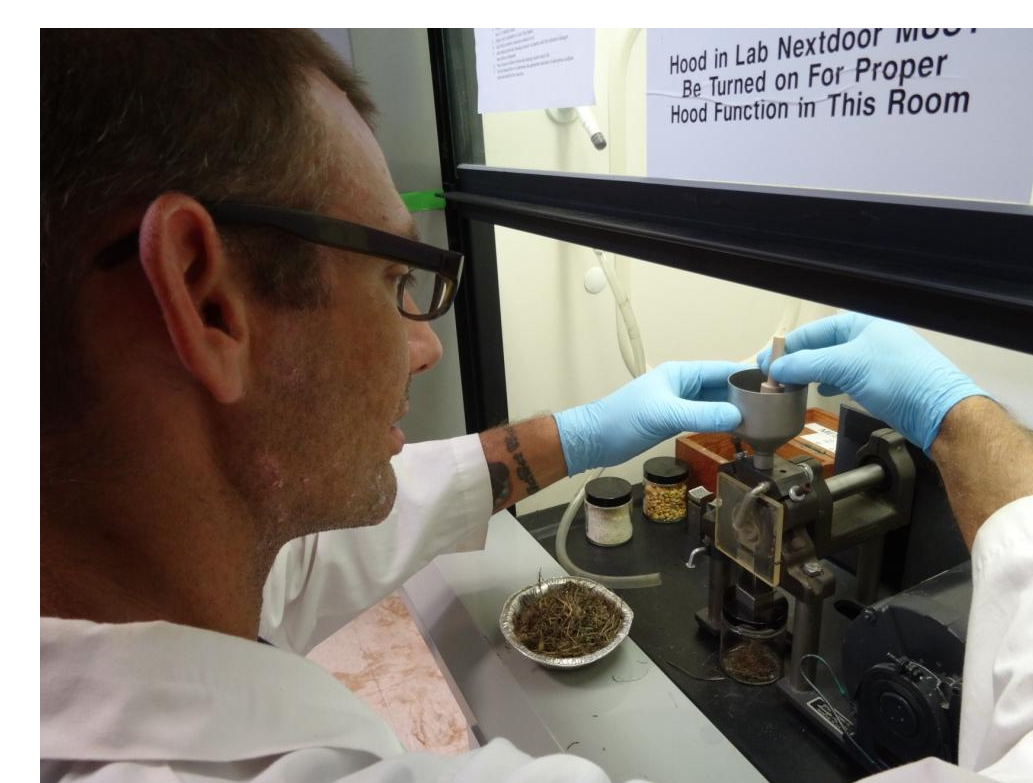
0.85 mm particle size achieved with Wiley mill
