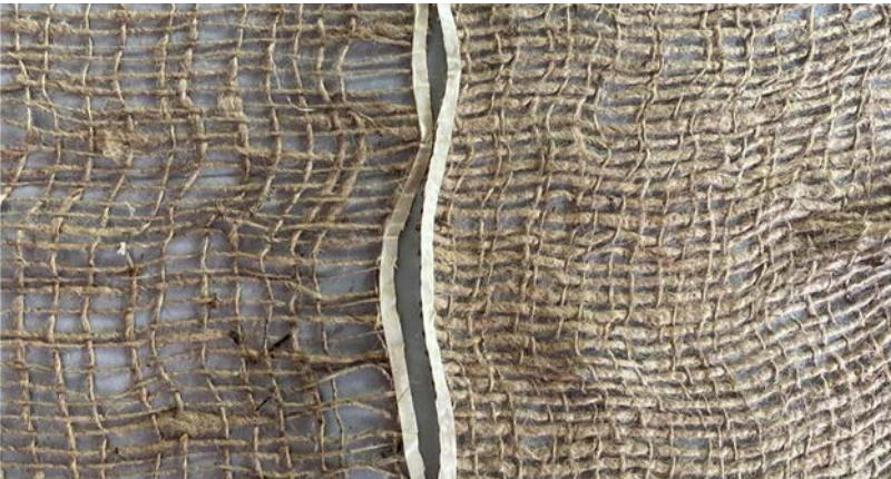
Figure C.1. Range in quality of jute erosion control mat. The matting pictured on the left side has a warp thread count of 21.3 threads ft-1 and a weft thread count of 9.7 threads ft-1 with a diameter of 3.6 and 4 mm respectively. On the right, matting shown has a warp thread count of 21.6 threads ft-1 and weft thread count of 14.0 threads ft-1 with thread diameters of 6.7 and 3.6 mm respectively.
