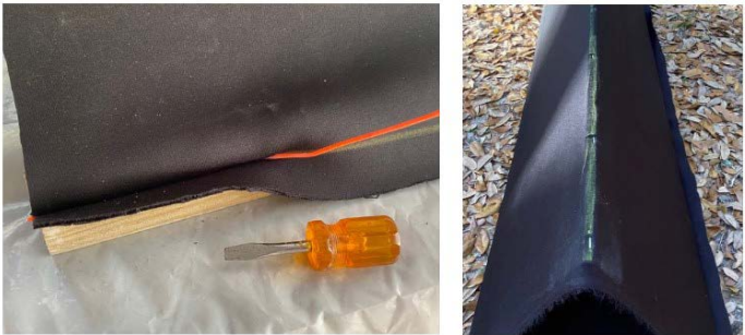
Pressing the spline into the fabric along the groove line (left) and stapling fabric to outer edge of rail (right).
