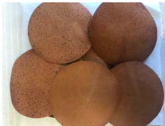
The final preparation step causes FeO strips to become a brown color. (Photo provided)
