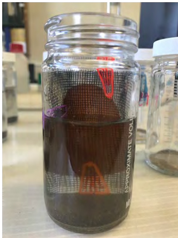
Protected FeO strips are placed in a glass bottle for P extraction. (Photo provided)
