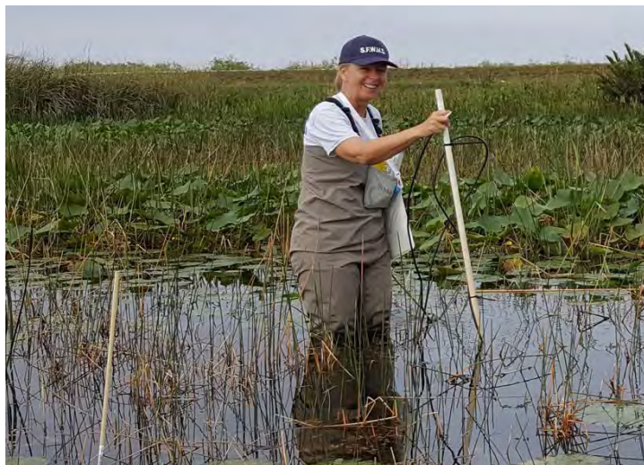
Measuring the effects of plant density on water velocity. (Photo provided)
