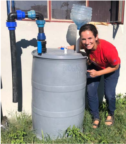
Claverie stands next to her anaerobic digester. All the materials were locally sourced, and she built the digester with her team. (Photo provided)
