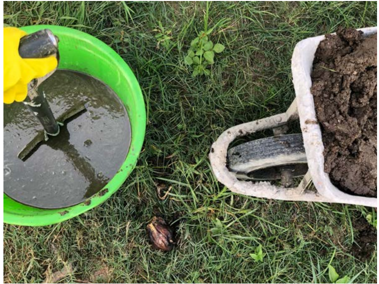
To build the microbiome in the anaerobic digester, Claverie added a mix of manure from the local village and water. (Photo provided)
