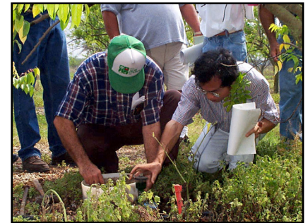
Yuncong Li shows a Homestead grower how tensiometers can help schedule irrigation.
