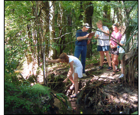
Mark Clark shows county extension agents how to measure stream flow and calculate pollutant loads.
