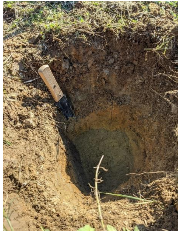
Figure 2: Right: Photograph taken from the Northern edge of the field that shows the M horizon at about 10 cm, and strong gleying at 40 cm.
