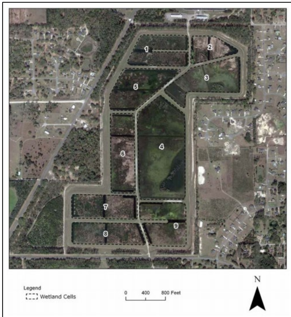
Figure 10: The Ichetucknee Sprayfield Treatment Wetlands. Secondary effluent flows through the nine cells, treating nitrogen and phosphorus-laden waters, which is ultimately ends in groundwater recharging cells. Source- Knight and Keller, 2019.'
